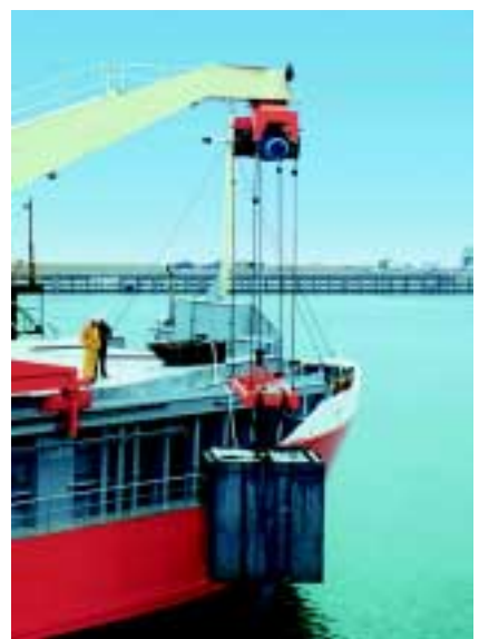
No load swinging: HÜBNER HOG 10 + ESL combinations (Digital-Tacho + electronic overspeed switch) control and monitor the movement of the AC brake motors.
