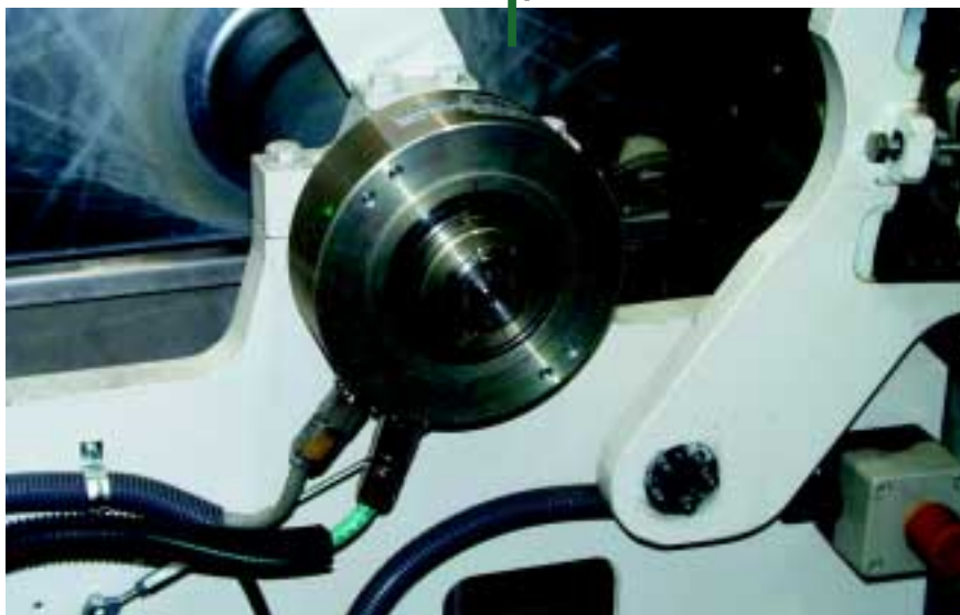
Positioning even in harsh environments: Bearing-less HÜBNER HG 18 Digital-Tachos measure and synchronize the speed of the drives on this vertical lift railway bridge near Rotterdam (➔ Figure 25 on page 19).
